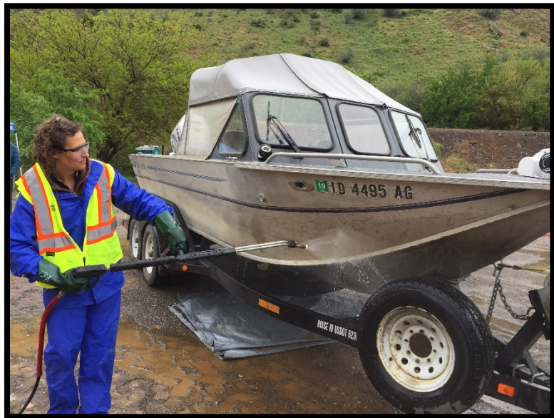
FIGURE 7 IDAHO DEPARTMENT OF AGRICULTURE INSPECTION STAFF DEMONSTRATING DECONTAMINATION OF TYPICAL ON-SITE WATERCRAFT
